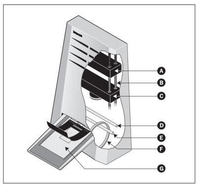
Figure 3: Cut-away view of Flextight 646
